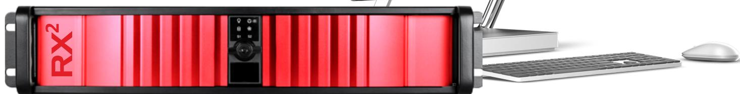
Cinedeck's RX2 redesign features a rack mountable, slim 2U chassis that can record 2i/2o or 4in mode. Cinedeck's UI, Client 2.0 provides even greater flexibility for your production and can run independently as a controller, scheduler or multiviewer on any Mac or PC device, controlling one or more Cinedeck appliances.
